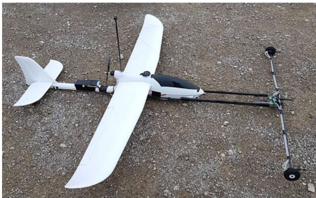
Fig. 7 UAS testbed with three 5-hole probes connected to high-dynamic differential pressure sensors
