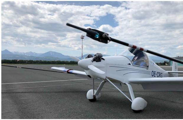
Fig. 9 Manned experimental aircraft with 5-hole probe and differential pressure sensors in front of the wing
